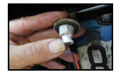
Plug in the new led strip aligning the red with brown and black with black. Turn on the lights and test. If it doesn't light, unplug and turn it 180 degrees and plug it in. Re-test.
