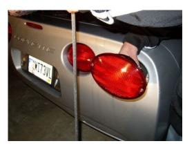
Peel the adhesive backing (yellow strip) off the seal. Starting at the top or bottom of the taillight, gently press the seal onto the tail light all the way around the perimeter. You want the big side of the seal facing OUT and the thin side facing the front of your car.
