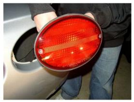
Gently slide the tail light back into the bumper and screw in the Torx screws. Repeat for each tail light
